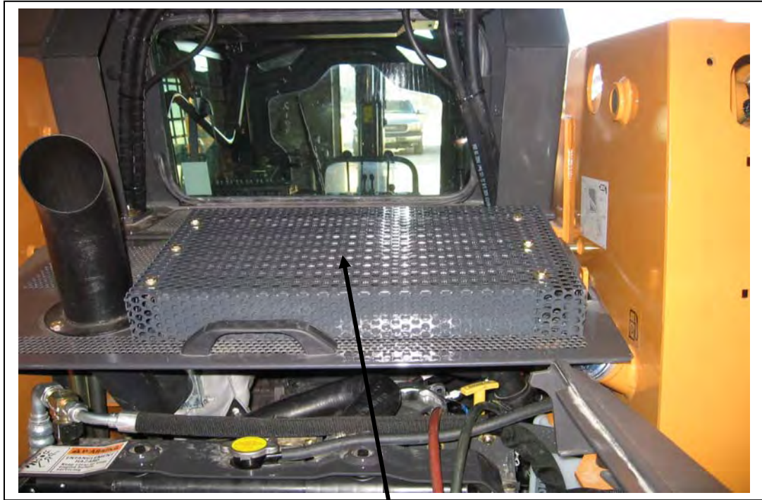
Condenser in place with engine cover closed.
