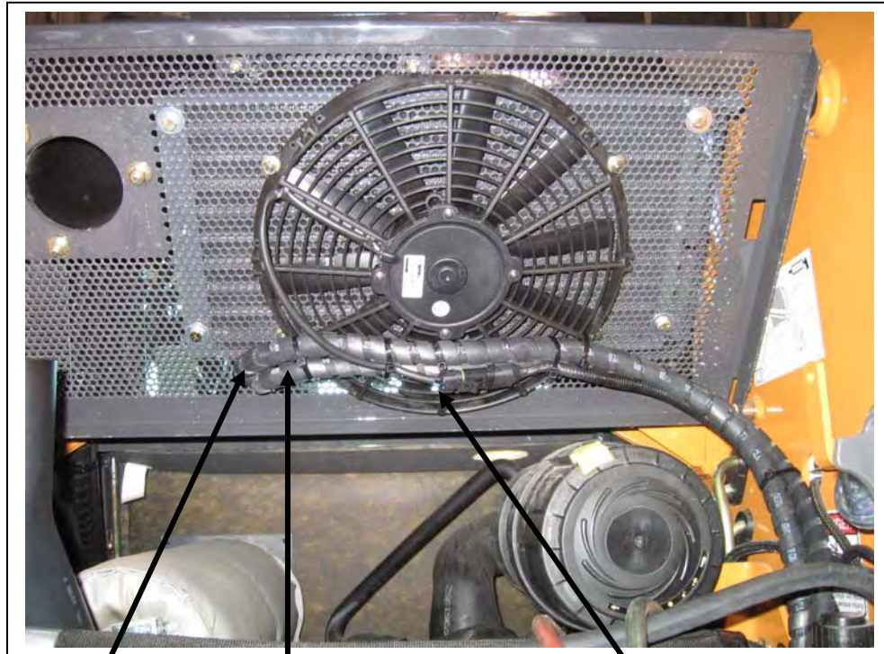
Electrical connection at condenser fan. If fan pushes out instead of pulling in, reverse the wires.
